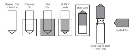
The "dwell" time in the latex determines the latex pick-up or thickness for each dip. A single dip can produce a wall gauge from .005" to .025". A multiple dip process is used for wall gauges greater than .025". Very heavy parts are possible (over .1"), but tolerances are difficult to maintain, especially if the part is long.
