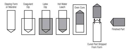
The "dwell" time in the latex determines the latex pick-up or thickness for each dip. A single dip can produce a wall gauge from .005" to .025". A multiple dip process is used for wall gauges greater than .025". Very heavy parts are possible (over .1"), but tolerances are difficult to maintain, especially if the part is long.
